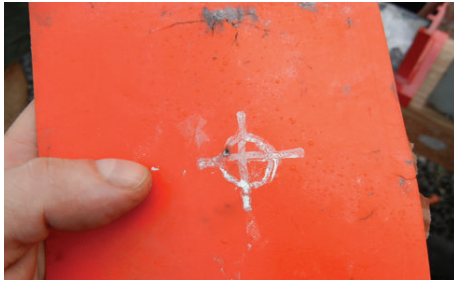
FIGURE 6: View of the hole caused by the shot over the plate of polyurethane.
